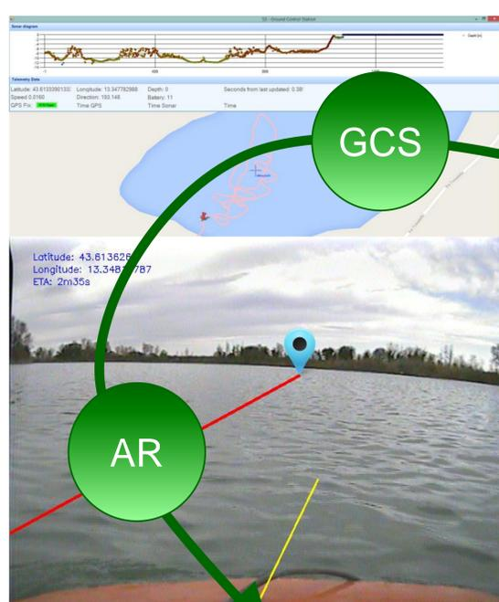
Augmented Reality (AR) app for a Smart control of survey. The desired waypoint is shown to the user as planned and actual path.
