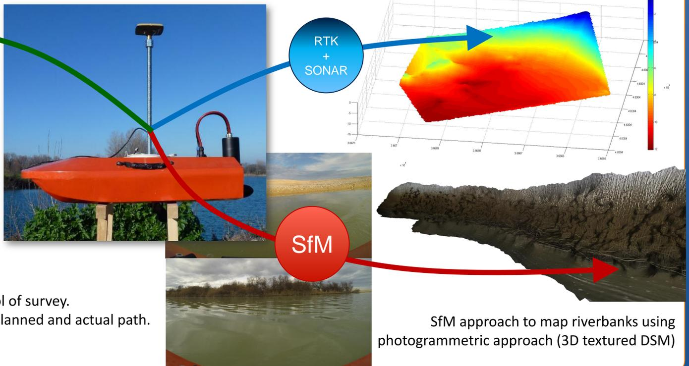
SfM approach to map riverbanks using photogrammetric approach (3D textured DSM)
