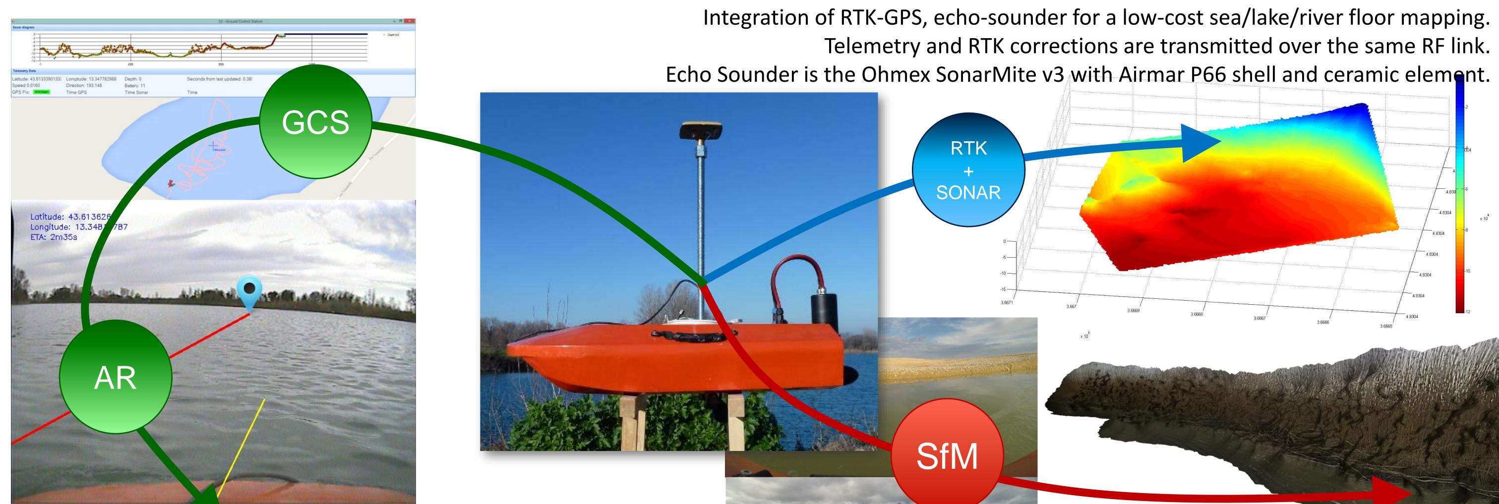
Augmented Reality (AR) app for a Smart control of survey. The desired waypoint is shown to the user as planned and actual path.
